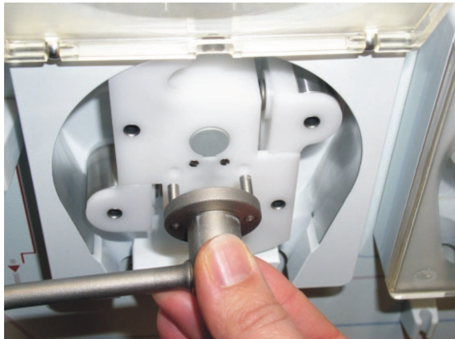
Fig. 13-3 Use of crank (alternative 2)
