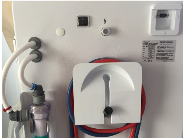
Fig. 4-1 Storage of cables and tubes
