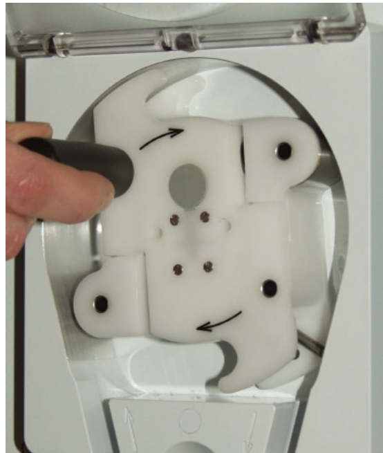
Fig. 13-2 Use of crank (alternative 1)
