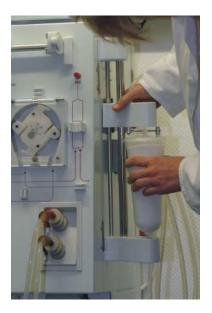
Fig. 11-22 Inserting a cartridge
