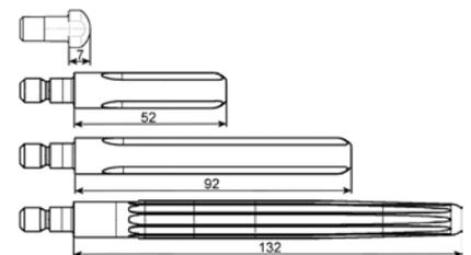
The overall length of the tibia plateau with the respective extension stem is given by the tibia keel length (dimension D) and the obturator 7 mm or the stem length 52, 92 or 132 mm.
