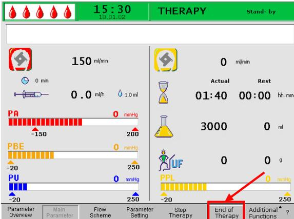
When the treated plasma volume is achieved, the machine switches to the stand-by mode. The blood circuit continues to circulate with the most recent blood flow rate selected.
