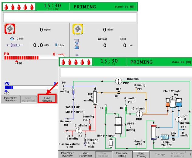
By selecting the **<Flow Scheme>** menu item in the menu bar, the display changes to the Flow Scheme. When in the **<Flow Scheme>** screen and the **<Parameter Setting>** menu item is selected in the menu bar, the screen changes to the Parameter Overview.
