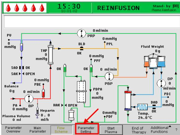
To set the parameters, select the **<Parameter Setting>** menu item with the cursor in the **<Flow Scheme>** screen and activate it with the
