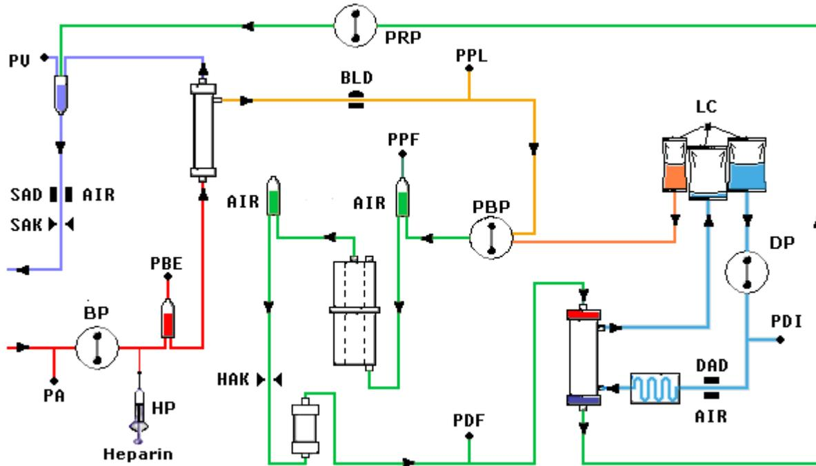
After the dialysis, the plasma is delivered via the reinfusion pump (PRP) to the venous air chamber and together with the blood from the plasma separation reinfused to the patient via the venous line.
