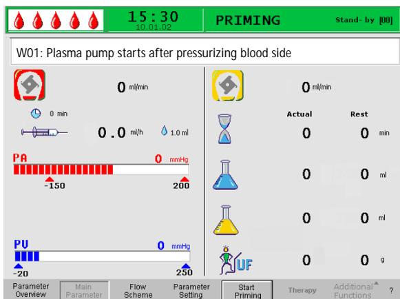
After starting priming by selecting **<Start Priming>**, the message **<W01: Plasma pump starts after pressurizing blood side>** is displayed in the message line.
