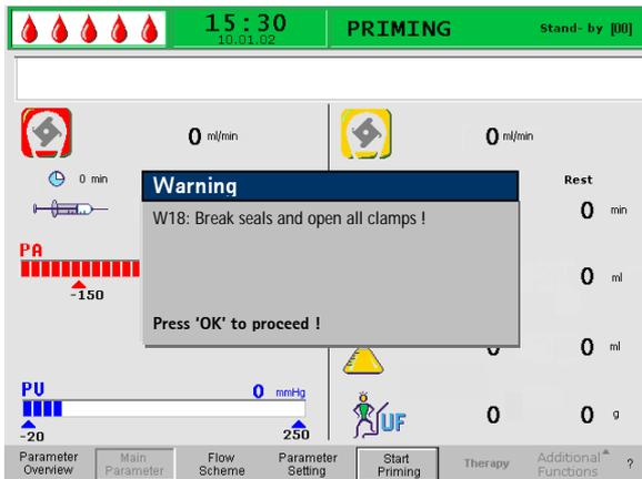
Warnings requiring an action are displayed in a Warning window, they must be acknowledged with the
