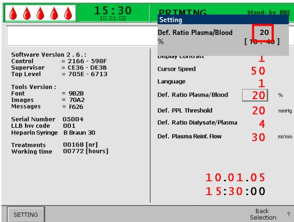
If a parameter is relevant to patient safety, the currently set value is shown in the Setting window above the setting range. In addition, the LEDs above
