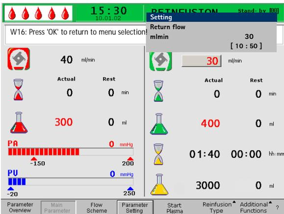
All parameters which can be changed are displayed in red. The currently selected parameter has a gray background. The Setting window displays the allowable range. Using the rotary knob, select the individual parameters.
