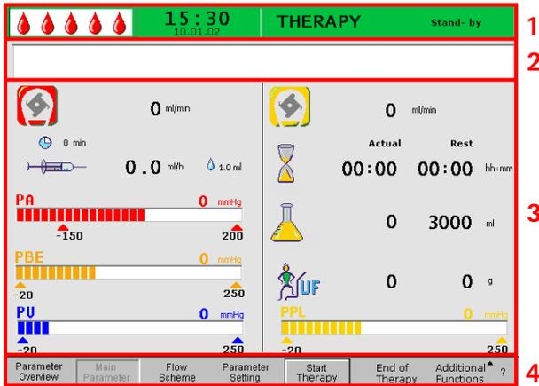
1 **Status bar:** The status bar indicates the activity of the blood pump, the current time and date, therapy phase (priming, therapy, reinfusion) and current status of the phase (stand by, running).
