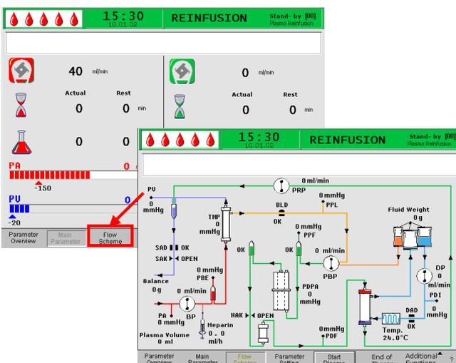
Using the rotary knob and the
