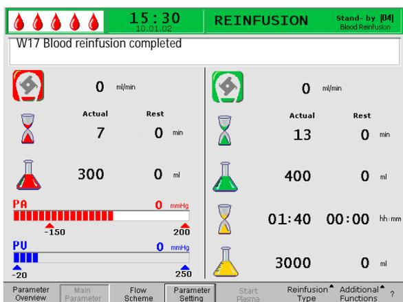
The blood pump stops automatically when the set blood reinfusion volume is reached.
