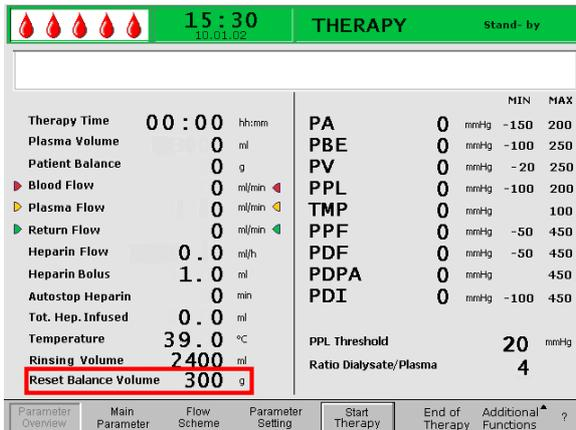
During a balance reset, the load cell is newly tared. The data of the balance reset are saved and shown in the Parameter Overview. Every reset performed in the course of the therapy is saved and the values are summated.
