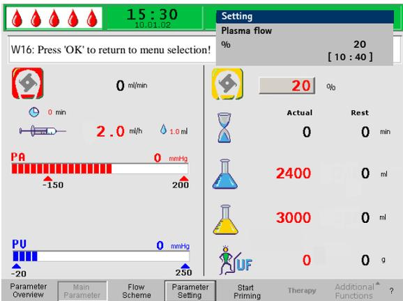
All parameters which can be changed are displayed in red. The currently selected parameter has a gray background. The range which can be selected is displayed in the Setting window. Using the rotary knob, you can select the individual parameters.
