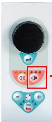
Alarm key with LEDs
