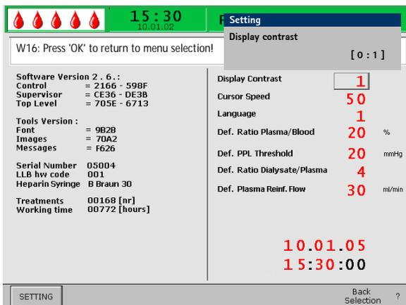
All parameters that can be changed are displayed in red. The currently selected parameter has a gray background. The Setting window displays the allowable range. Using the rotary knob, select the individual parameters.
