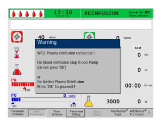
When the reinfusion volume is reached, all pumps except the blood pump stop. The blood flow is maintained. The default setting of the plasma reinfusion volume is 400 mL.
