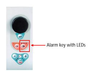
An active alarm is also indicated by the red LEDs
