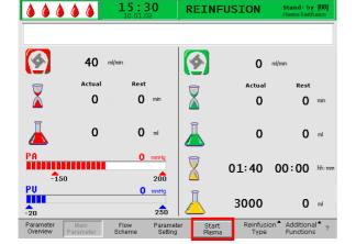
If the precipitate filter pressure rises during the plasma reinfusion because of the high filter saturation, the reinfusion flow should be reduced.
