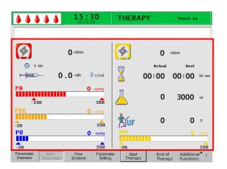
The change to the therapy phase is possible only when the minimum rinsing volume of 2400 ml has been reached.
