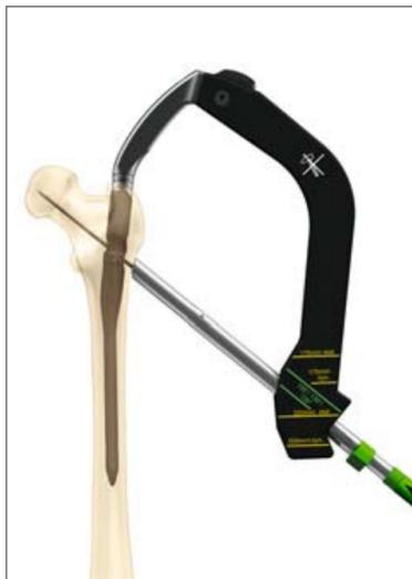
Drilling for TeleScrew drill bit remains in place
