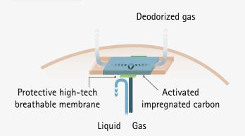
• Leak-Proof and permeable to gases high-tech breathable membrane
